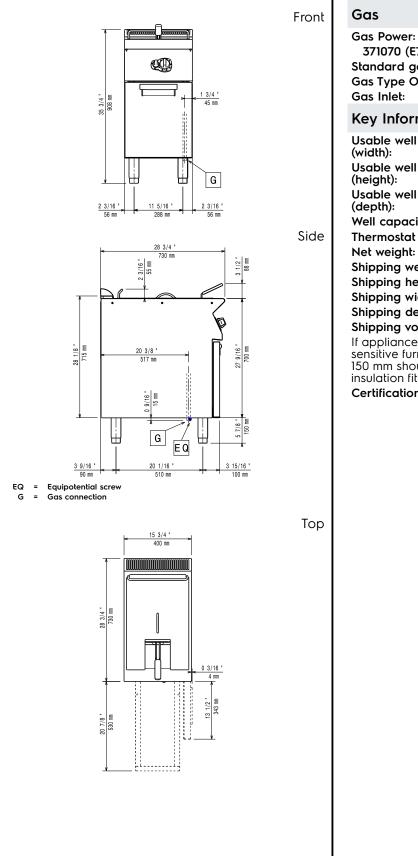
Standard gas delivery: Natural Gas G20 (20mbar) Gas Type Option: LPG;Natural Gas Gas Inlet: 1/2" **Key Information:** Usable well dimensions (width): 240 mm Usable well dimensions 505 mm (height): Usable well dimensions 380 mm (depth): Well capacity: 13 lt MIN; 15 lt MAX Thermostat Range: 105 °C MIN; 185 °C MAX Net weight: 55 kg Shipping weight: 58 kg Shipping height: 1140 mm Shipping width: 460 mm Shipping depth: 820 mm Shipping volume: 0.43 m<sup>3</sup>
